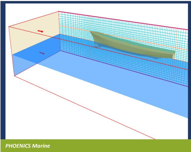
PHOENICS Marine will return values for drag, separated into skin friction and form drag, while displaying and quantifying size of bow and stern waves produced. An added innovation allows users to test their designs with sinusoidal waves as an input - see pg 11 of PHOENICS Newsletter Autumn 2017 for full description - and extract parameters such as pressure on the hull as a function of time. PHOENICS Marine users will benefit from current
