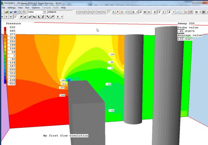
Lines separating the contour bands can be labelled automatically or manually.
