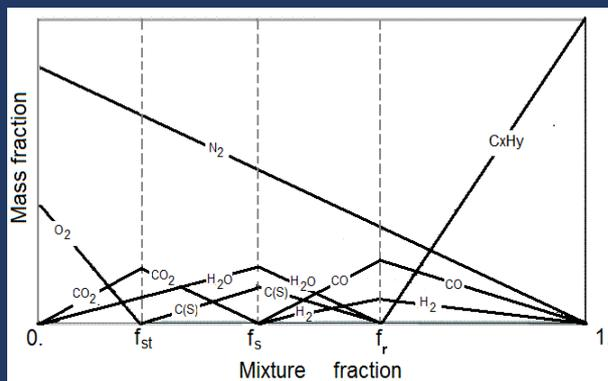
*Mixing and flame-limit discretization of reactions between fuel and oxidant streams producing soot, hydrogen and carbon monoxide intermediates [5]*
