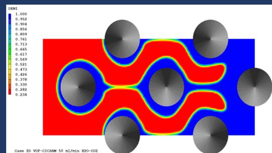
*Near Critical CO<sub>2</sub> Flowing in a Channel with Octagonal Micro-pillars filled with water.*
