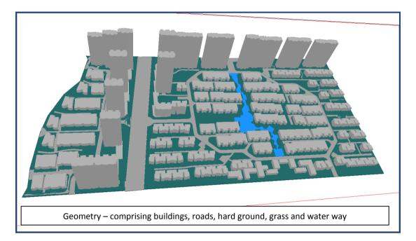
The idealised geometry shown above contains many of the components of interest to the "Heatisle" engineer; viz, concrete and glass high rise buildings, tarmac roadways, hard terrain and vegetation, and a water course. Each component responds differently to solar radiation.
