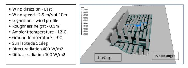
In this example, the ground surrounding the buildings, road, grass and river all have a Z depth of 2m. The ground temperature of 9°C is applied at the lower face of the ground. This represents the constant earth temperature underground.
