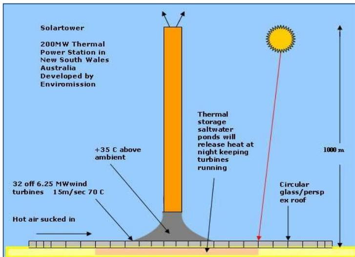
A Solar Updraft Tower is a relatively low cost, low tech, renewable energy system for generating electricity from solar power.
