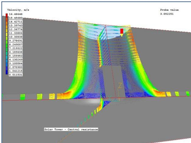
InForm is used to apply the heat sources to hidden blockages, HEAT & HEAT2. The STOREd variable MARK is set to 1 in all cells which are fluid and have a solid above them (i.e. on the next Z plane). Fluid cells are identified as having the property marker PRPS < 100, and solid cells as having PRPS > 99. The heat is then applied to all cells with MARK=1.
