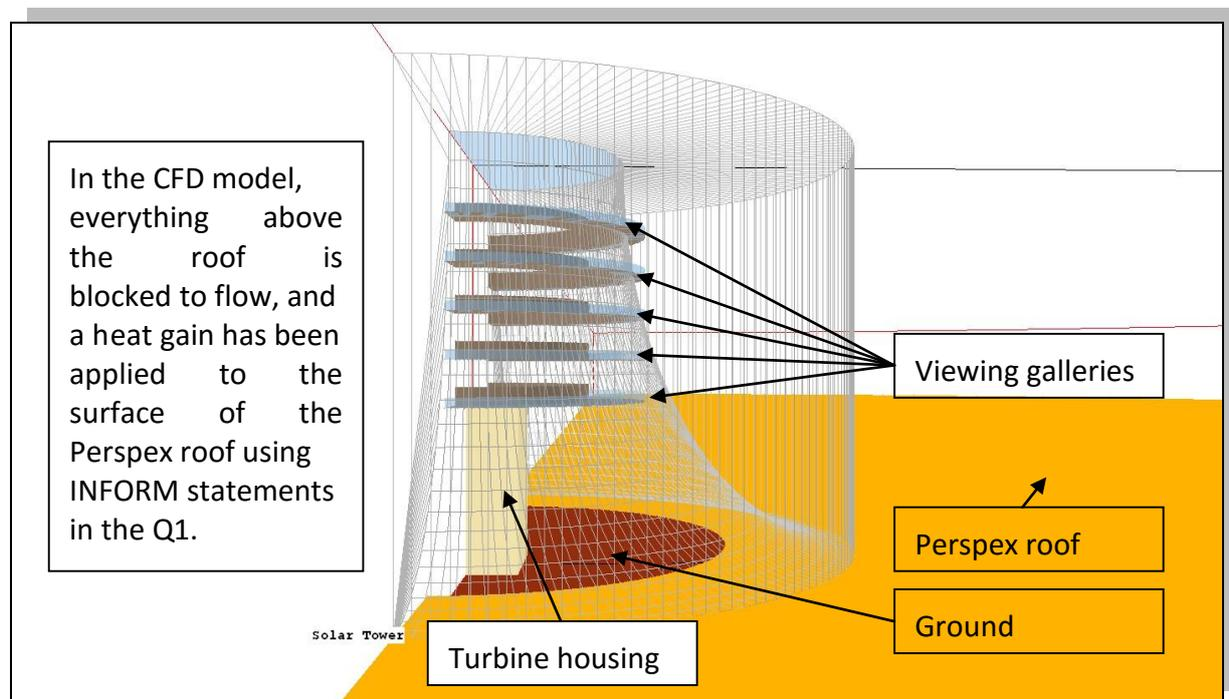
The image shows the inside of the tower. There are 5 floors inside with viewing galleries, each with a wall at the inner end and an ANGLED-OUT at the outer edge. The ANGLEDOUTs intersect the blockage of the tower and provide fixed-pressure boundaries where they intersect.
