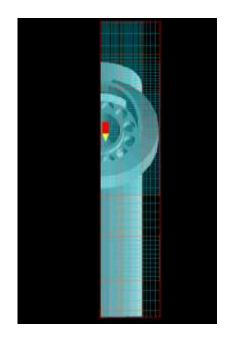
As can be seen, grid has been concentrated in the region of the nozzle and holes, and also where the inner pipe crosses the mesh at an angle.
