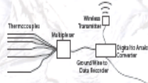
Figure 6 Diagram of field device. Main box will be filled with regolith simulant and embedded with thermocouples. Access will house electronics and shield them from access heat. b) Device electronics. Thermocouple data is combined to one channel by multiplexer, which sends signal to converter. Data transmitted through hardware and wireless signal to data recorder.
