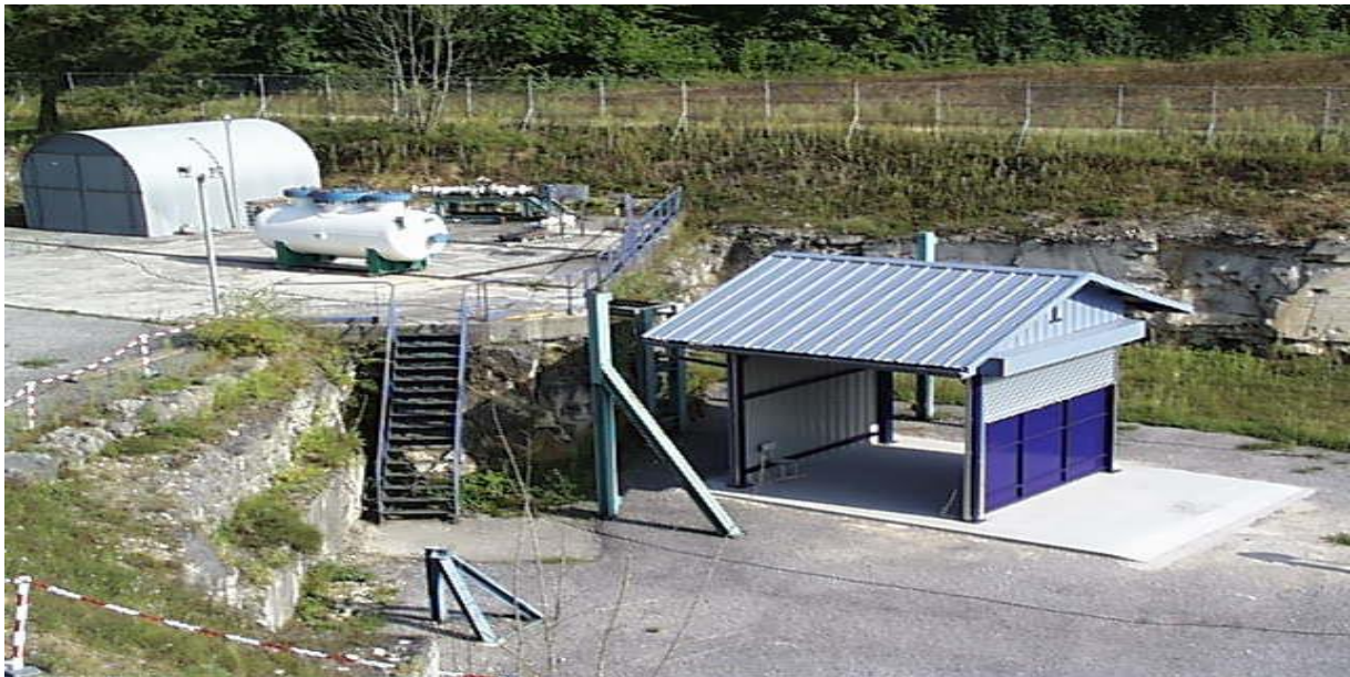
Fig 1 Surrounding of the experimental setup. Inside the cabin is vertical stud connected to the Butane (propane) tank from where a jet is coming to the ambient air. The blue wall is removed for the free jet case.
