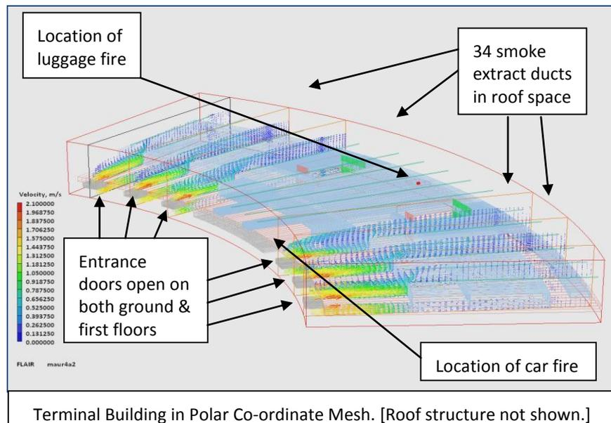
Transient calculations were needed to show the accumulation and dissipation of smoke product, its layering and the expected visibility at head height, throughout the progression of each fire simulated. As before, the CFD model incorporated operation of the smoke
